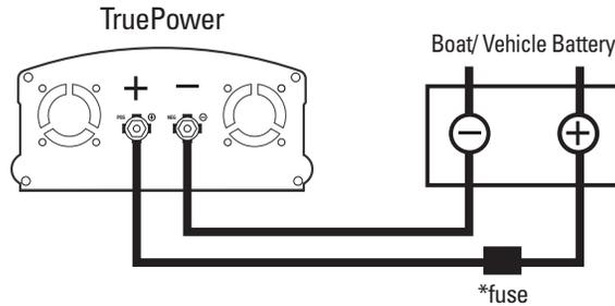
*\*For an ABYC E-11 compliant installation, customer supplied fuse, 7" from battery*
